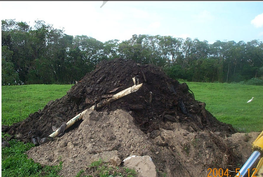
Photograph 3 Pit 4. Concrete, PVC pipe, and organic waste.
