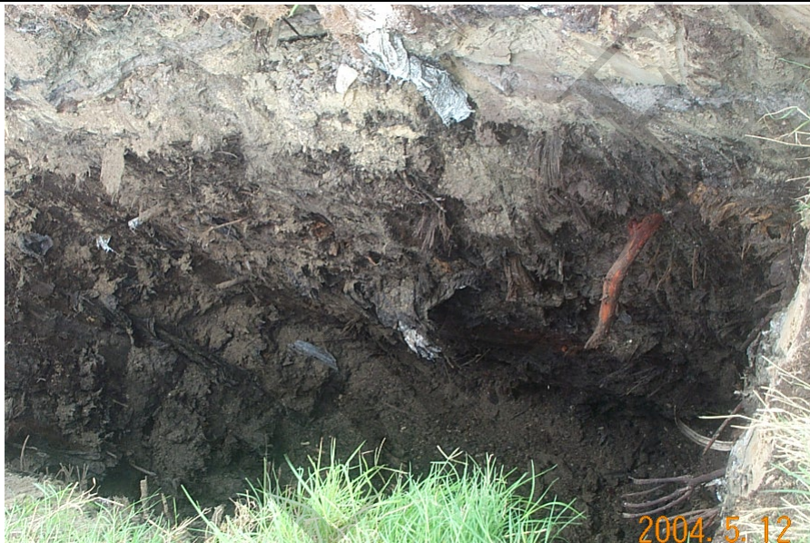
Photograph 2 Pit 1. Excavation sidewalls showing organic waste and plastic.
